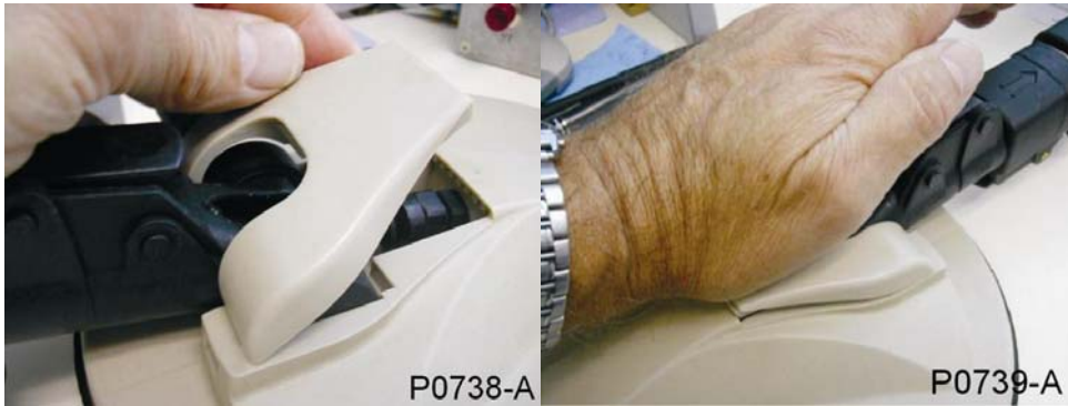
Figure 23: Fitting the Coil Retainer
