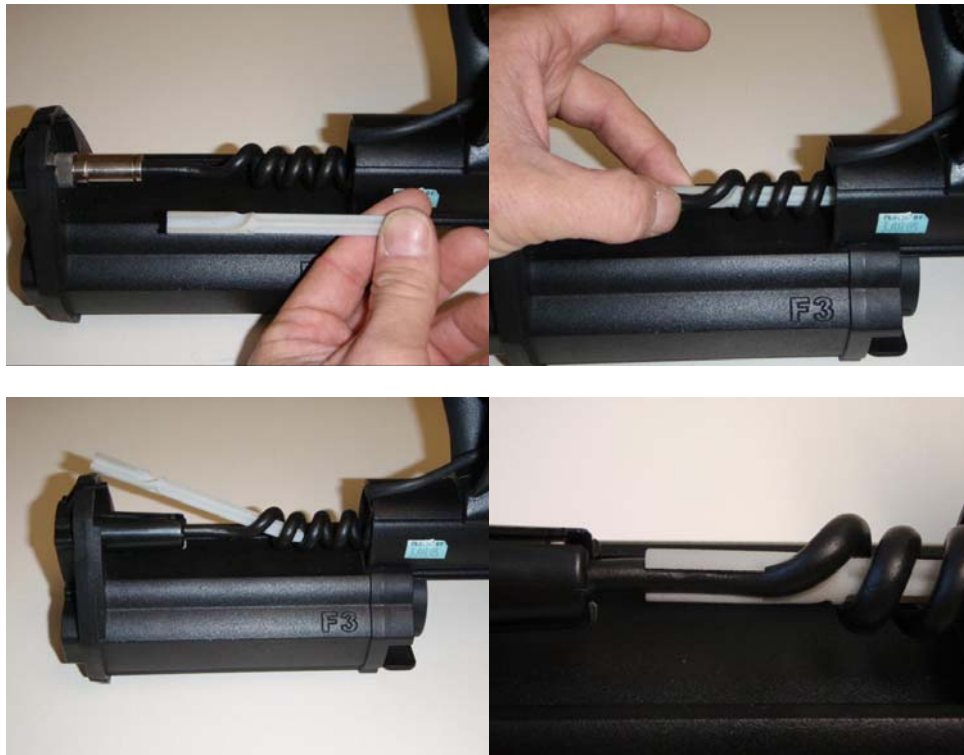
Figure 17: Inserting the Coil Pin
