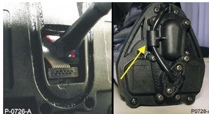
Figure 13: Excess Wiring Loom Cable Folded Correctly & Cable Router
