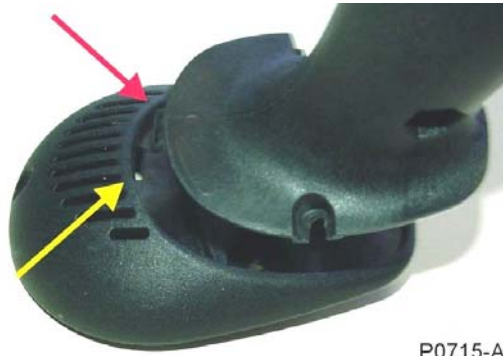
Figure 27: Fitting Speaker Pod onto Handle
