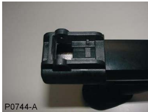
Figure 48: Upper Camlock Positioned on Upper Shaft
